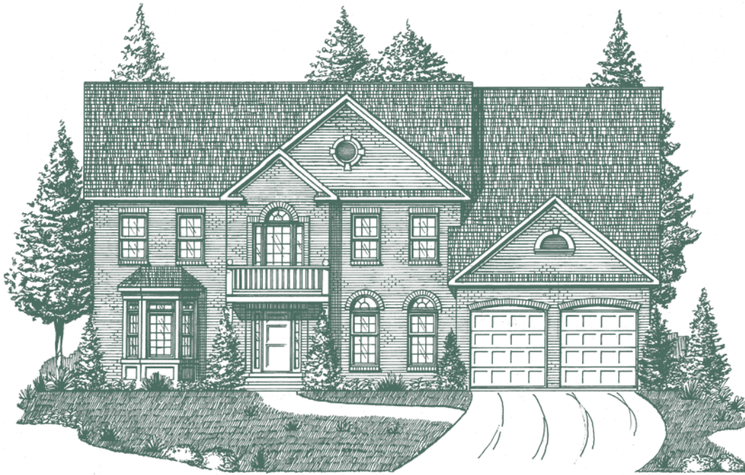
Elevation I with Optional Portico and Bay in Living Room, Siding Standard over Garage Reverse Gable and Siding over Large Reverse Gable on Main House
